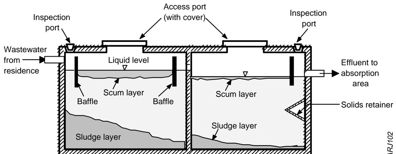
Figure 2. Cross-section of a typical two-chamber septic tank.
